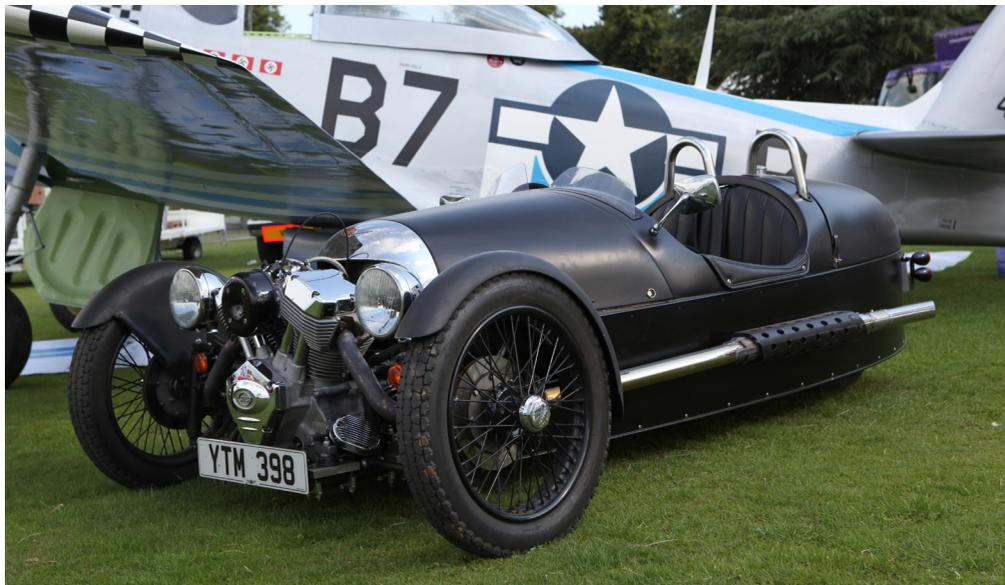
the engine is counterbalanced by the mass of the passengers and the car has a planted feel with a very low centre of gravity to ensure it remains super-glued to the road.
