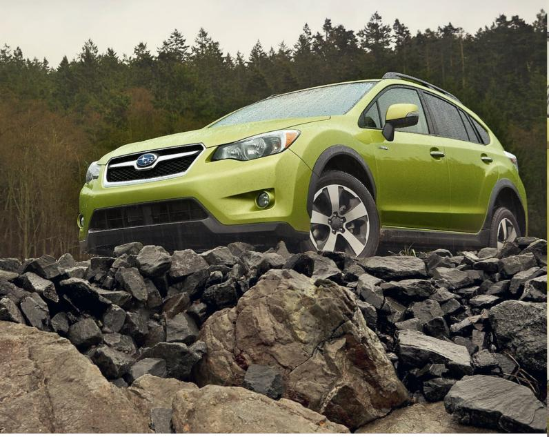
Every XV is equipped with Symmetrical All-Wheel Drive and a Boxer engine – ensuring an engaging and dependable drive in all conditions. Despite a ground clearance of 220mm, the Sport Utility Vehicle (SUV) offers a low centre of gravity, which aids its "on-road" grip, and helps it to achieve 0-62mph in 9.3 seconds.
