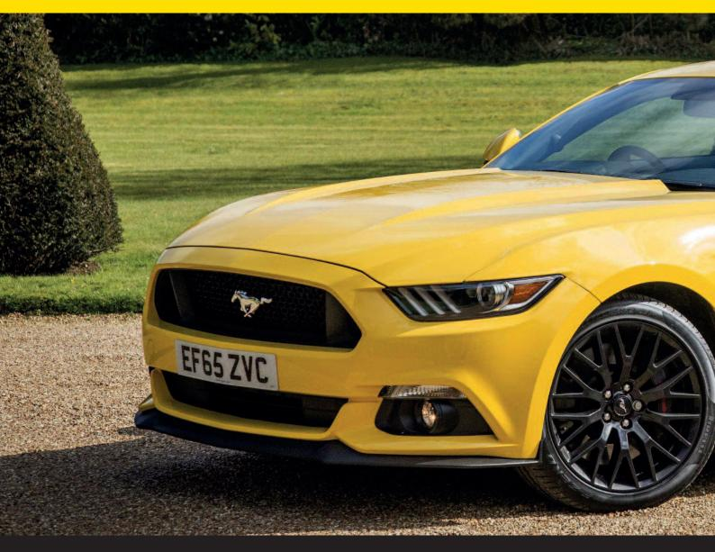
The Ford Mustang is presented with a 5.0-litre V8 block, or a fuel-efficient 2.3litre EcoBoost engine. The 5.0-litre fastback with six-speed manual transmission does the zero to 62mph sprint in 4.8sec - quicker than any Ford coupé in Europe since the limited Ford GT supercar came out over ten years ago. The Ford Mustang 2.3-litre EcoBoost fastback manual does the 0-62mph time in 5.8sec.
